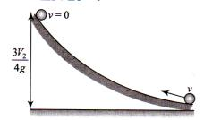
$$\left[0 - \left(\frac{1}{2}I\omega^2 + \frac{1}{2}mv^2\right)\right] + \left(mg \times \frac{3v^2}{4g}\right) = 0$$
